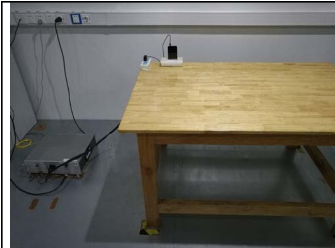
Conducted Emissions Test Setup Front View
