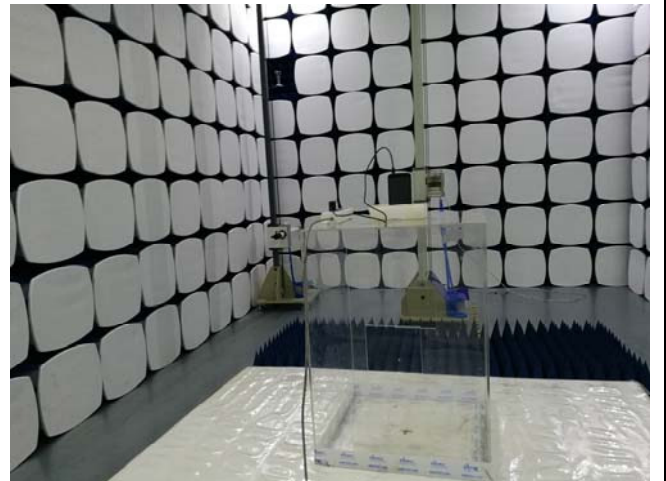
Radiated Spurious Emissions Test Setup Above 1GHz
