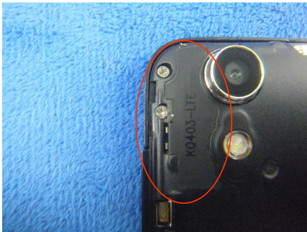
LTE - Antenna View
