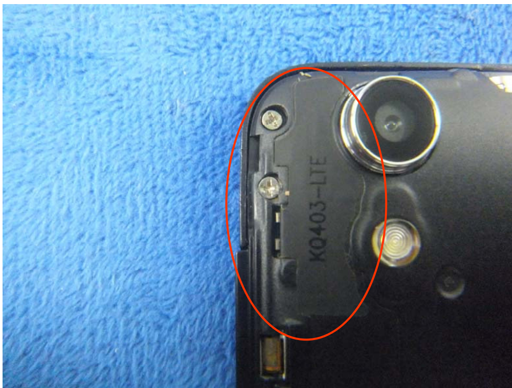
LTE - Antenna View
