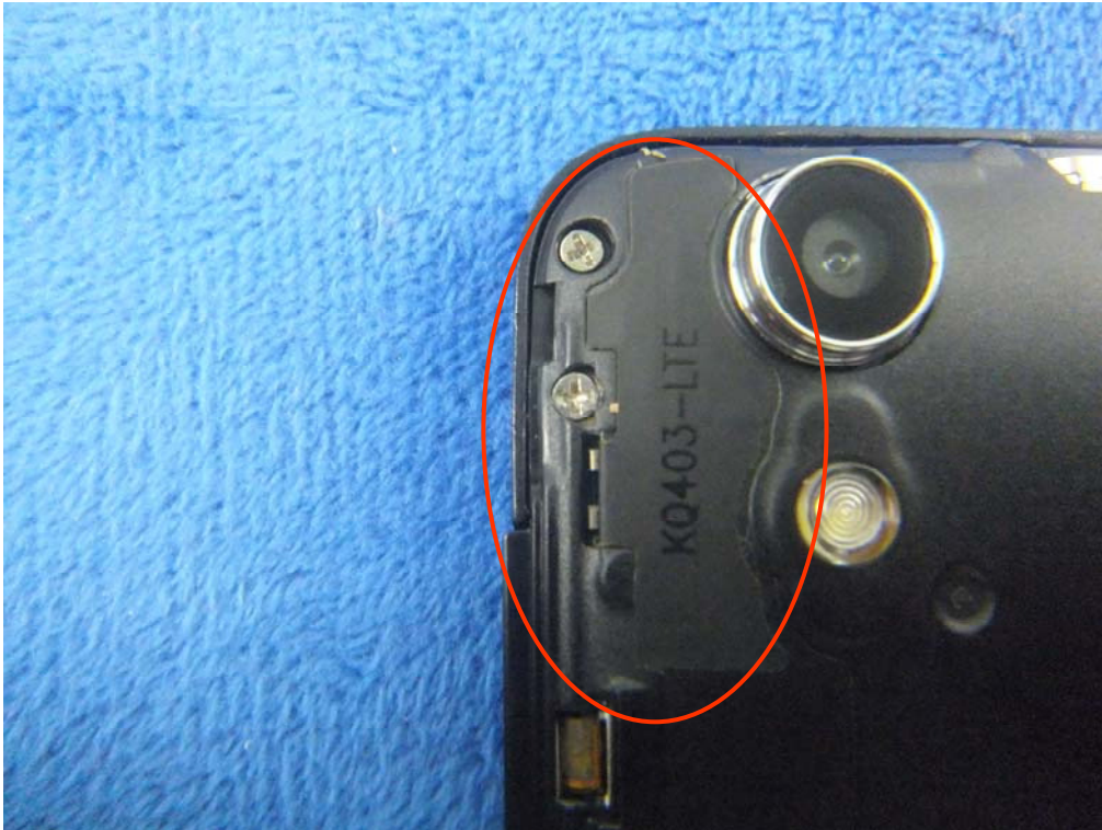
LTE - Antenna View
