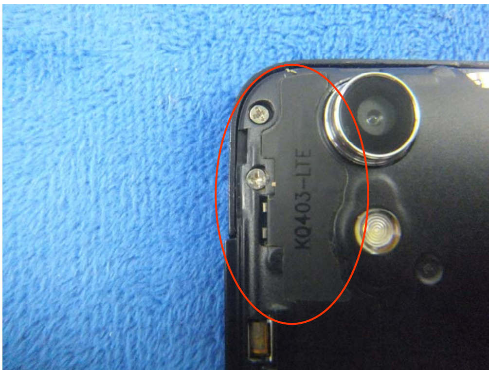
LTE - Antenna View
