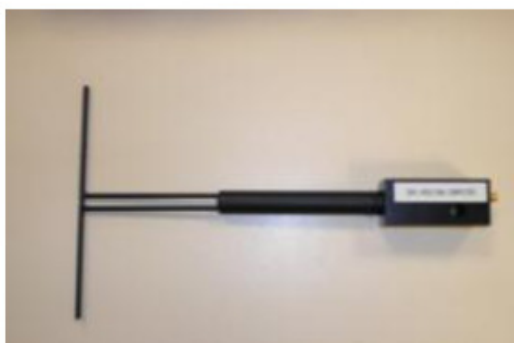
Figure 1 – Satimo COMOSAR Validation Dipole
