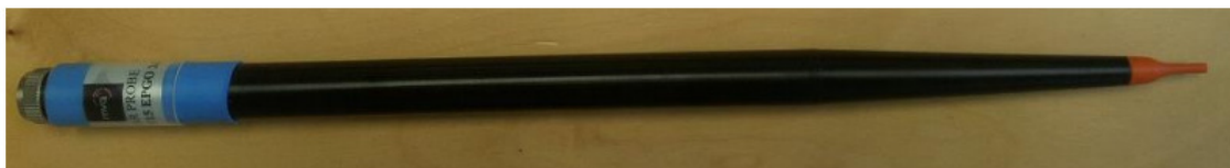
Figure 1 – MVG COMOSAR Dosimetric E field Dipole
