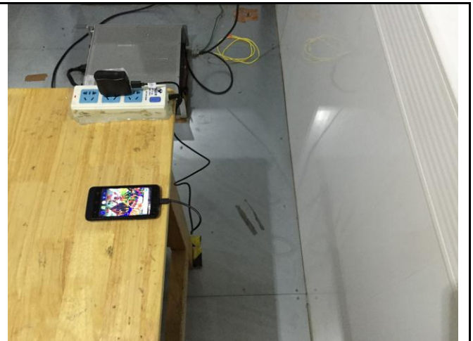
Conducted Emissions Test Setup Side View
