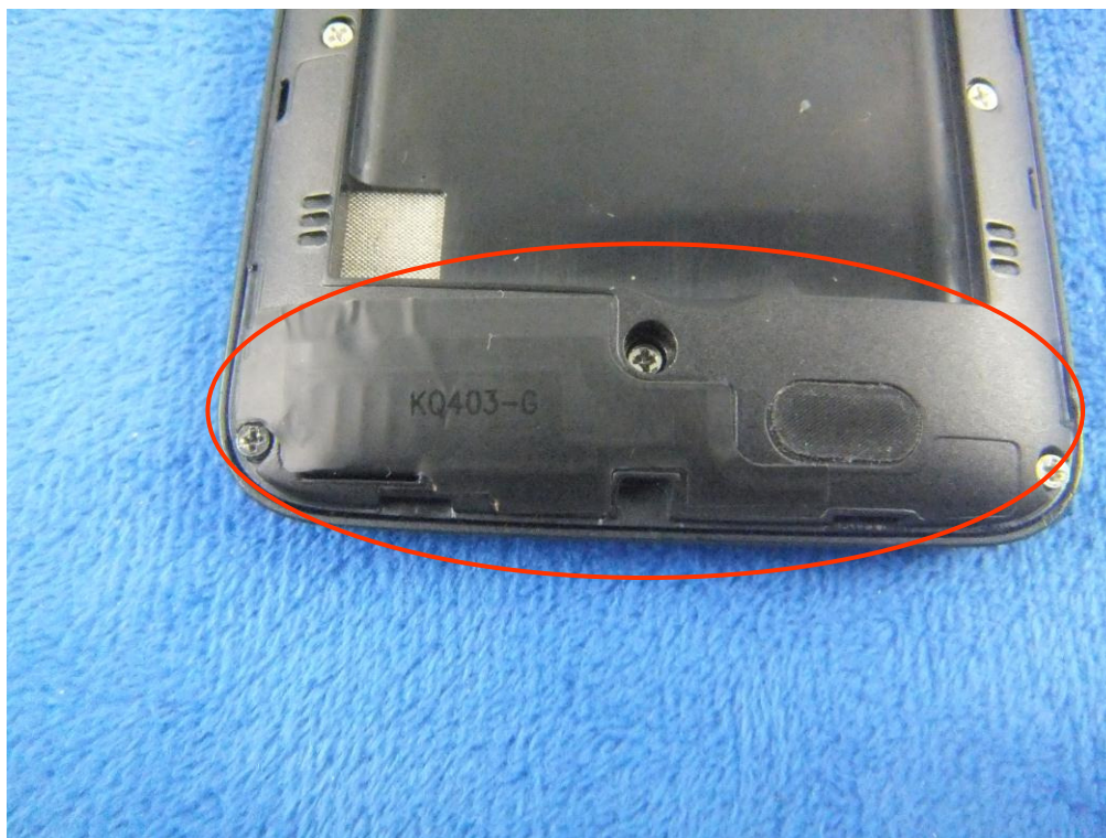
GSM/PCS/UMTS-FDD Antenna View
