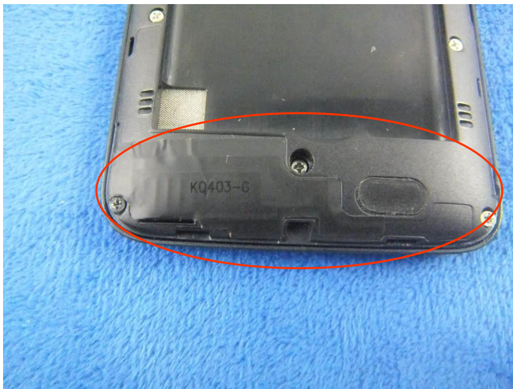
GSM/PCS/UMTS-FDD Antenna View
