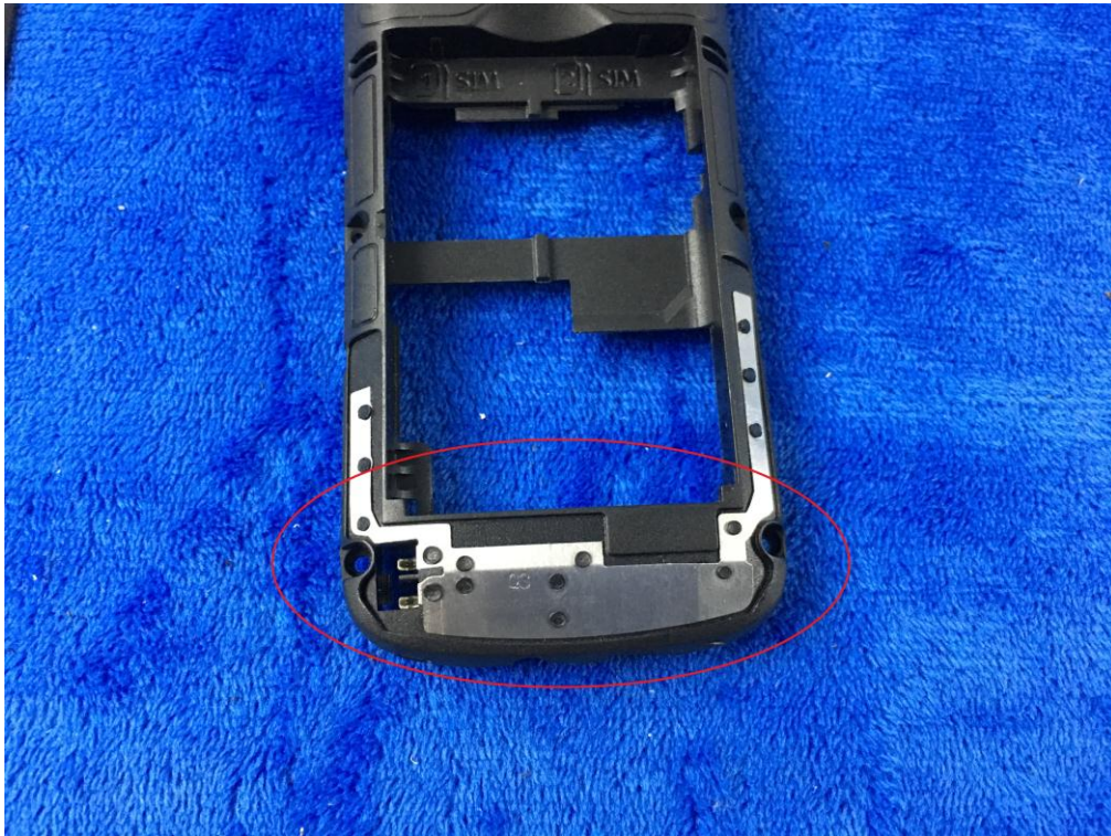
GSM/PCS Antenna View
