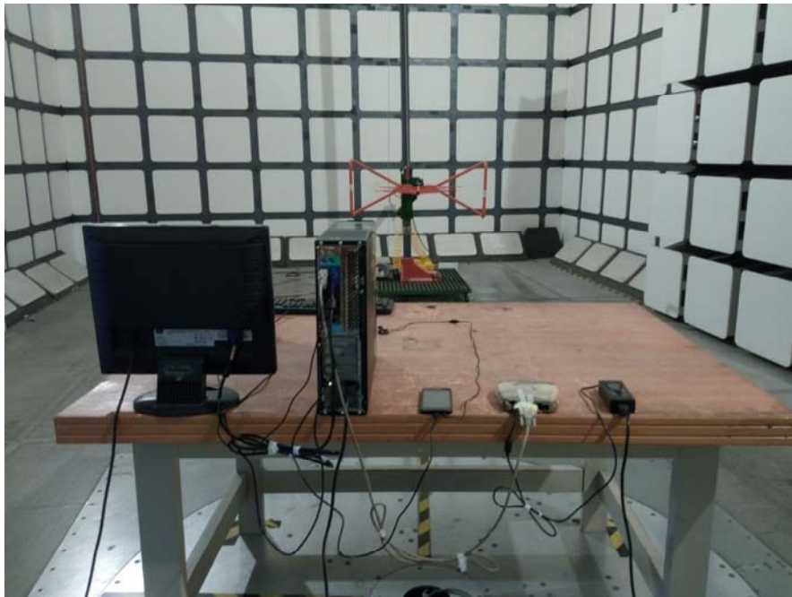
Radiated Emissions – Rear View (Below 1 GHz)
