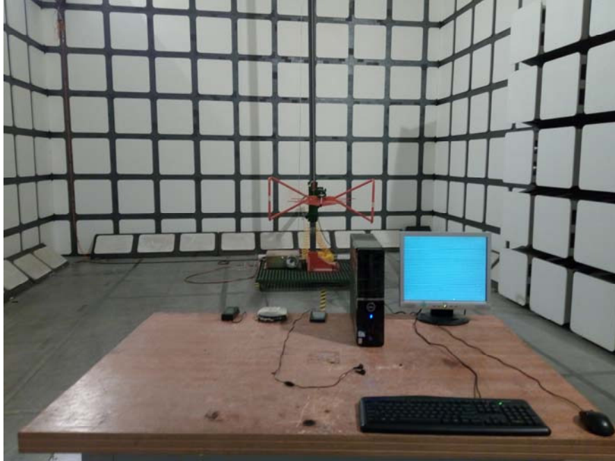
Radiated Emissions – Front View (Below 1 GHz)
