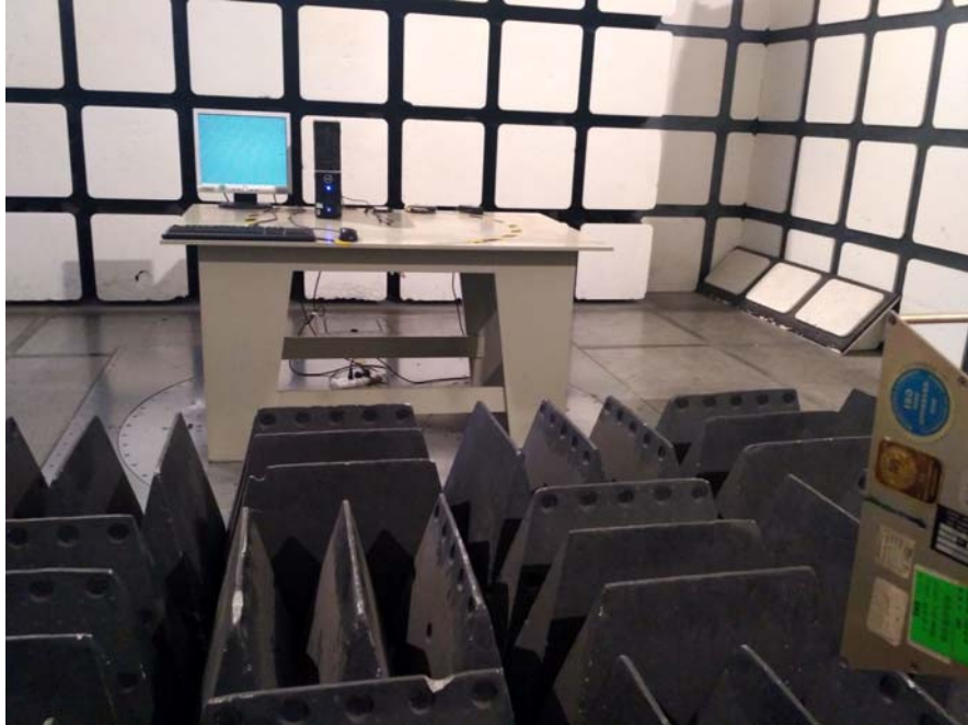
Radiated Emissions – Front View (Above 1 GHz)
