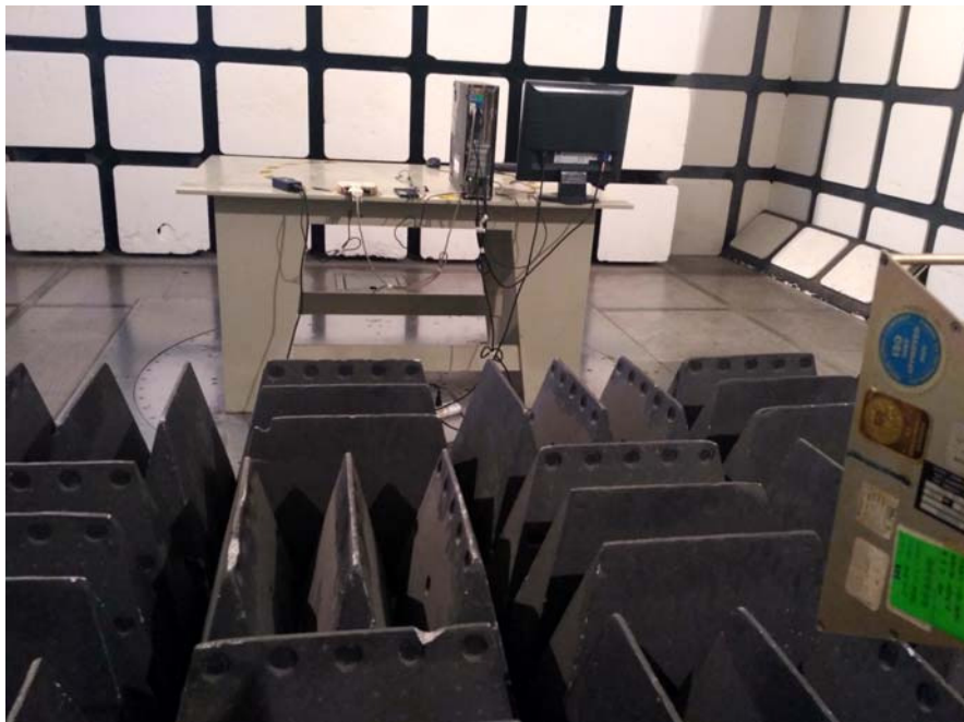
Radiated Emissions – Rear View (Above 1 GHz)
