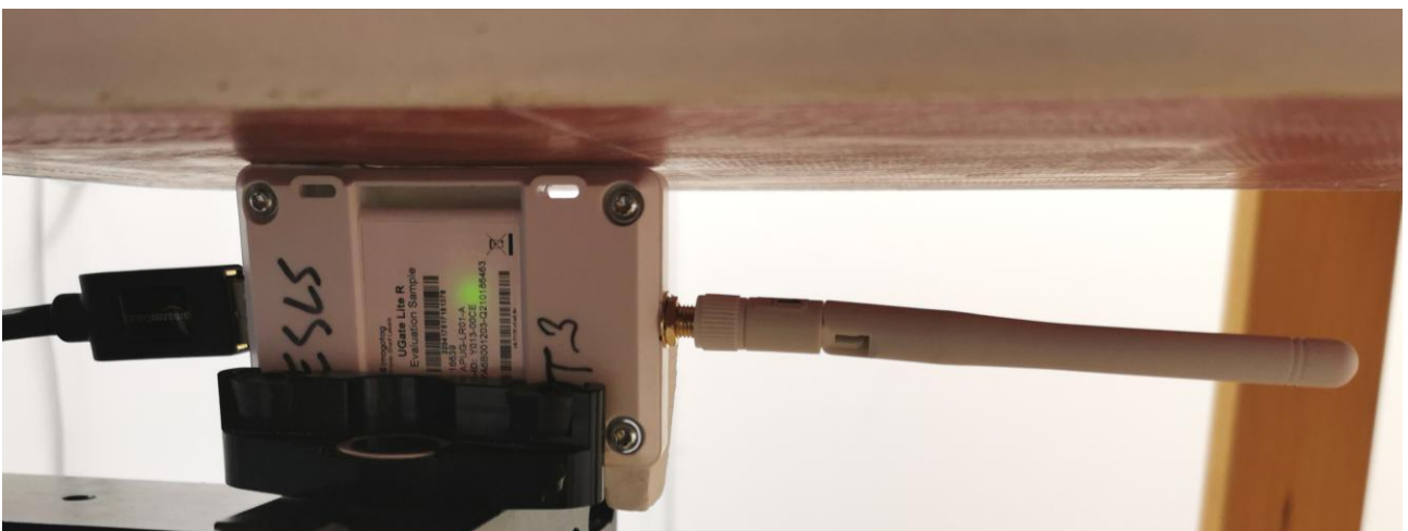
Figure 9 The left side of the device against the phantom, antenna straight
