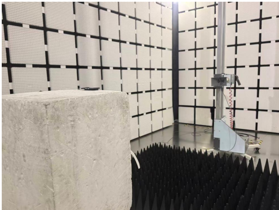
Photograph 2: Set-up for Radiated Spurious Emission, 1GHz - 18GHz
