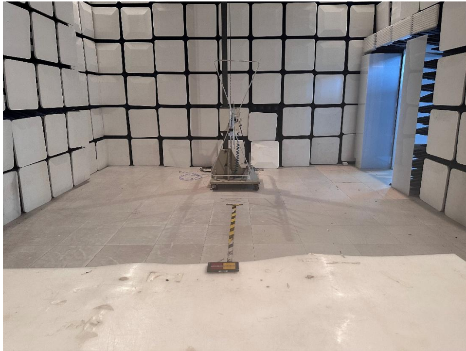
Photograph 1: Set-up for Radiated Spurious Emission, 30MHz - 1GHz
