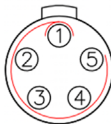
Figure 7 HJ394 C Port Welding Surface View
