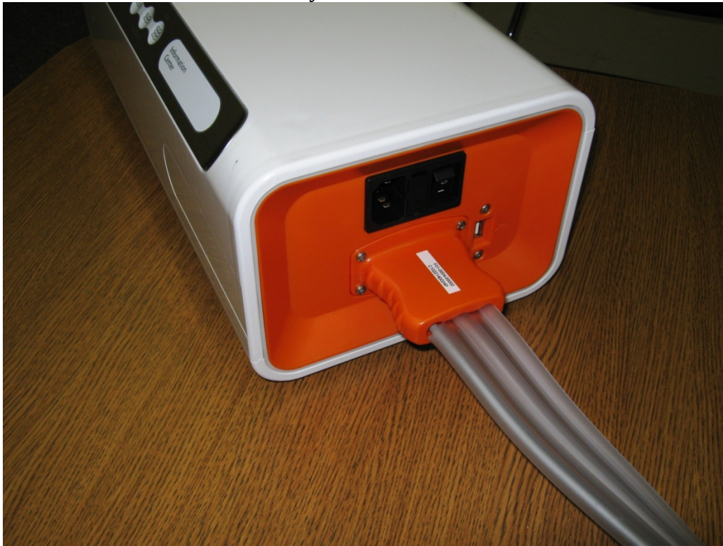
Hose Assembly connected to Controller
