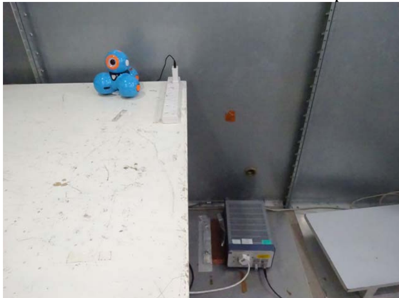
Measurement of Conducted Emission Test Set Up
