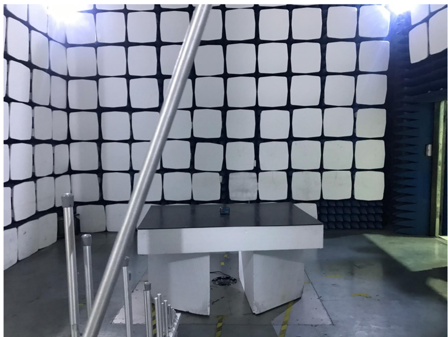
Radiation Emission Test Setup (30MHz to 1GHz)
