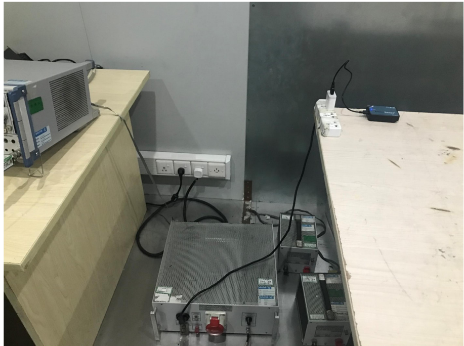
Conducted Emission Test Setup
