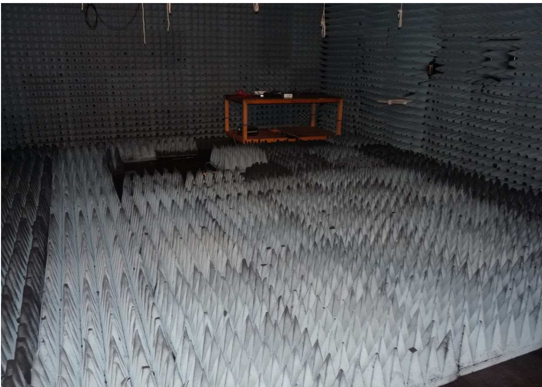
Photo 1: Test setup for radiated measurements, EUT in horizontal position Enclosure, semi-anechoic chamber, below 30 MHz, intentional radiator §15
