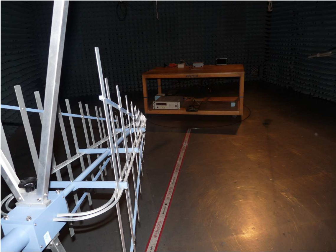
Photo 2: Test setup for radiated measurements, EUT in vertical position Enclosure, semi-anechoic chamber, 30 MHz to 1 GHz, intentional radiator §15
