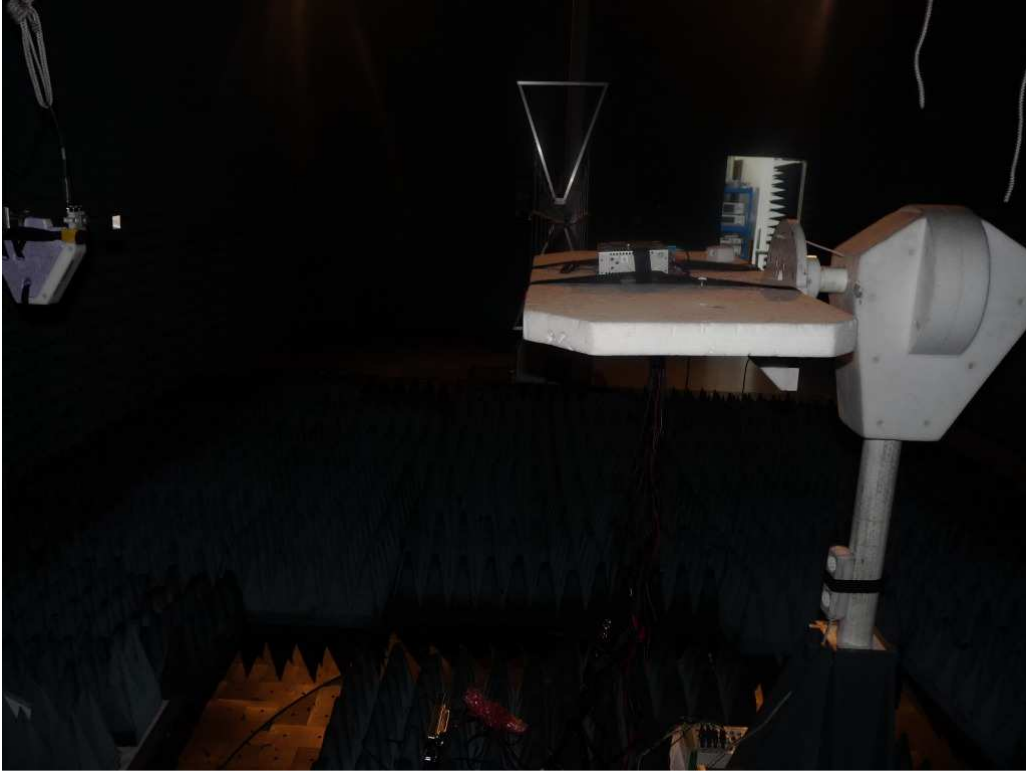
Photo 4: Test setup for radiated measurements, EUT in horizontal position Enclosure, fully-equipped anechoic chamber, 18-25 GHz. §15
