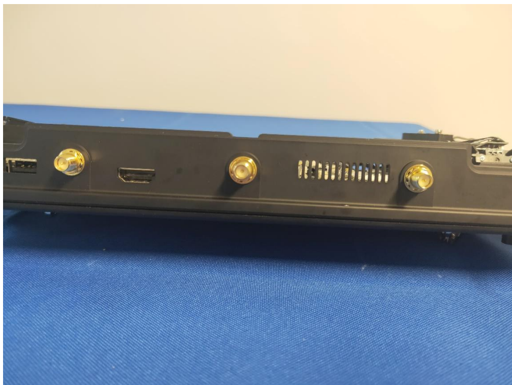
EUT UNCOVER VIEW (Antenna connector)
