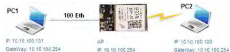
Figure 18. HF-A21-SMT Ethernet Interface Networking (As AP)
