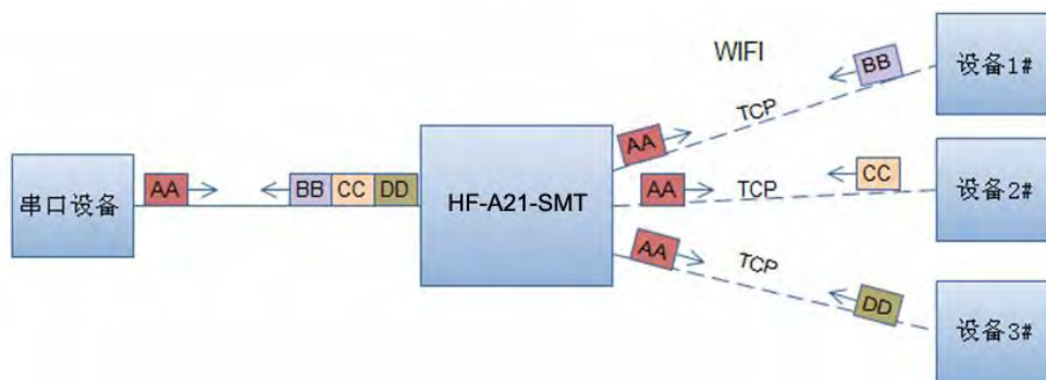
Figure 13. Multi-TCP Link Data Transmission Structure
