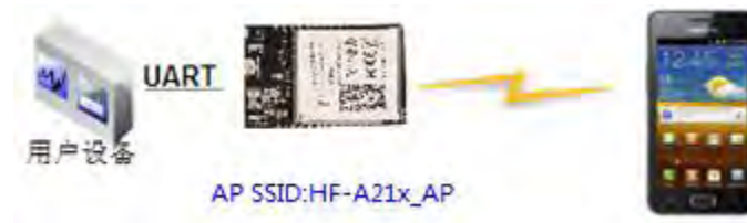
Figure 34. Wireless Control Application
