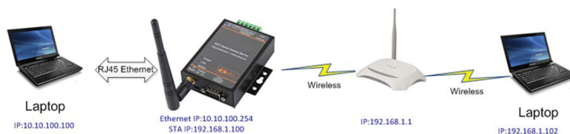
Figure 21. Ethernet Interface Function(Router)
