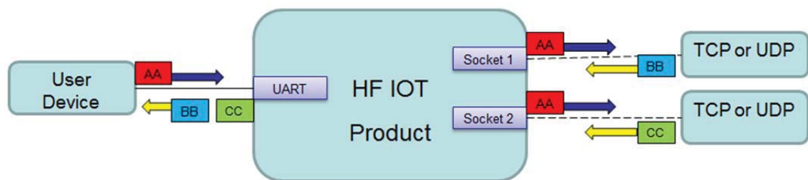
Figure 25. Multi Socket data transmission example
