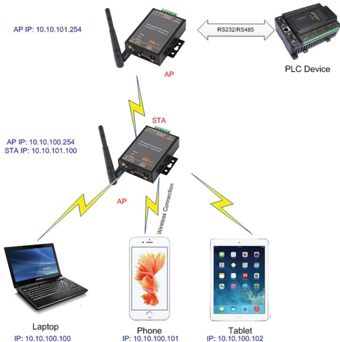
Figure 15. AP and STA Combination Application
