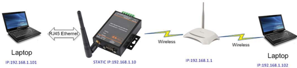
Figure 22. Ethernet Port Function(Bridge, reserved)
