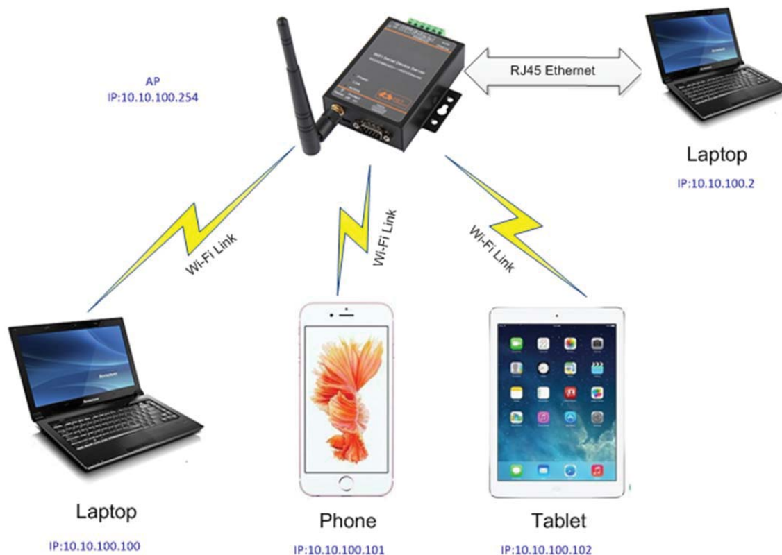
Figure 20. Ethernet Interface Function(AP)
