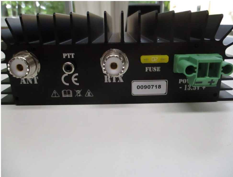
Photo A2-3: EUT, back, detail view
