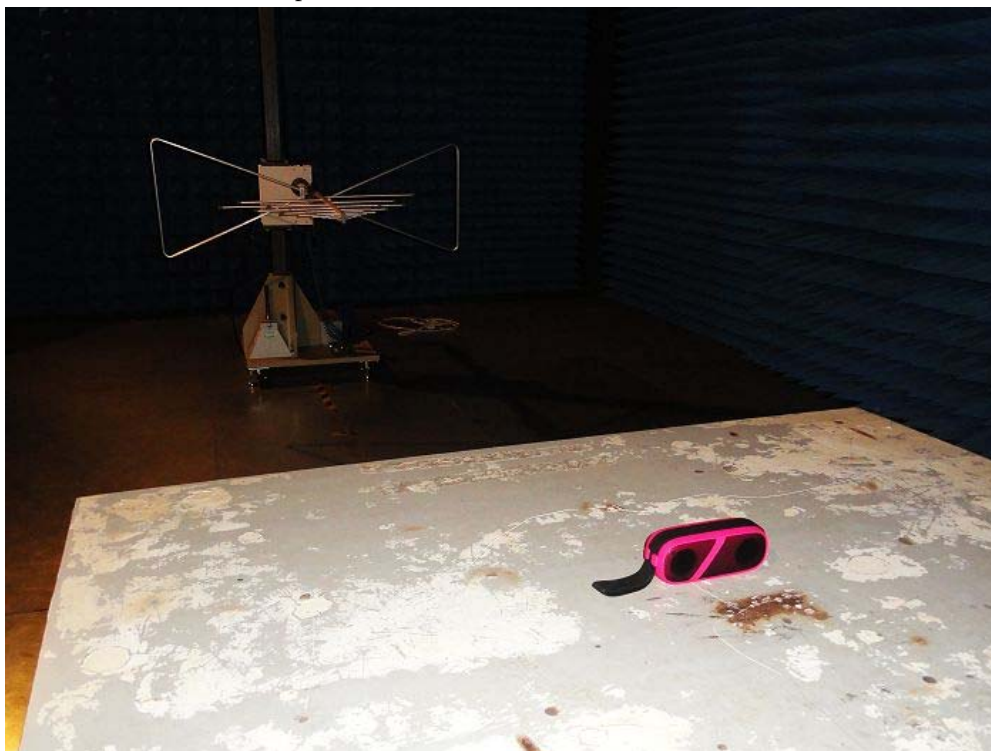
Radiated Emission Test Setup:
