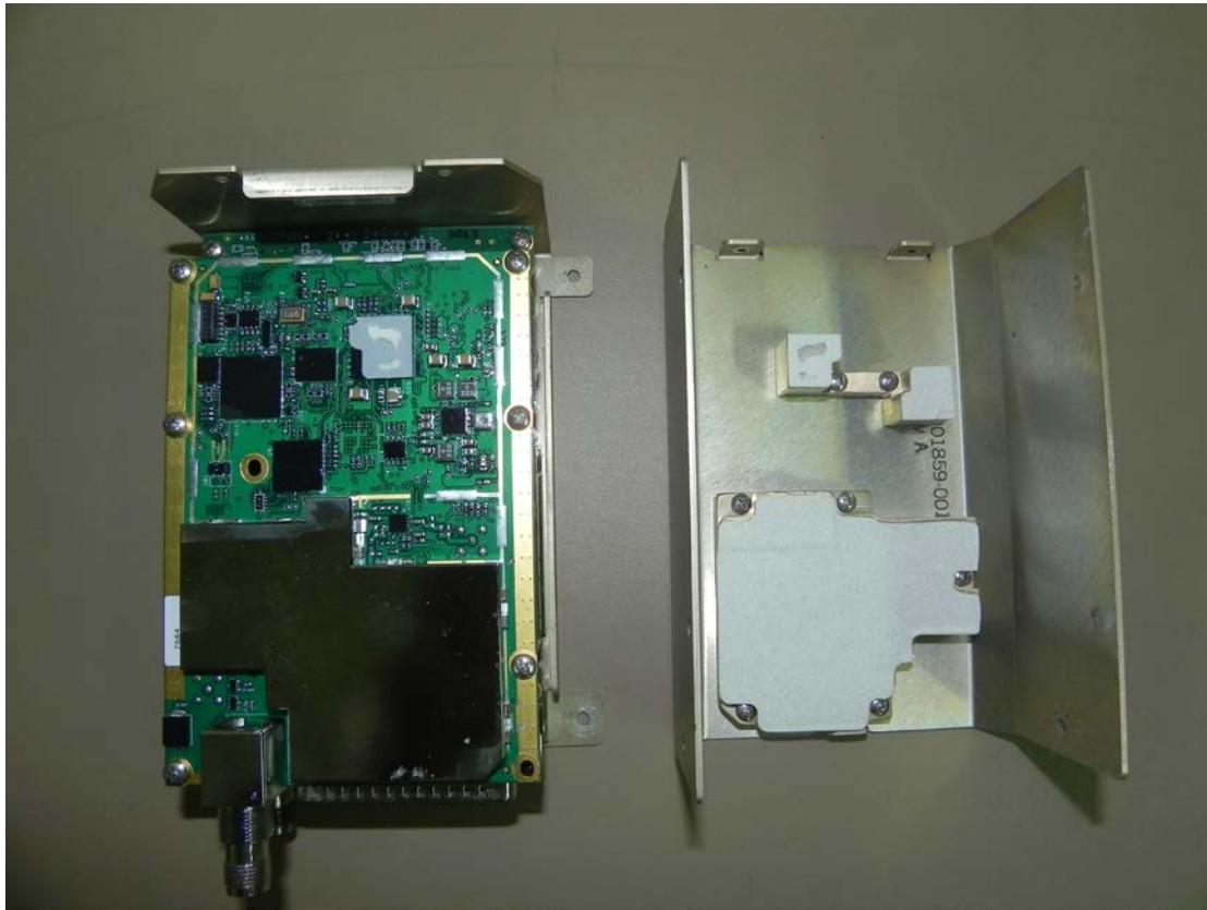
Figure 5-3: NGT-2500 Top View With Top Cover Removed
