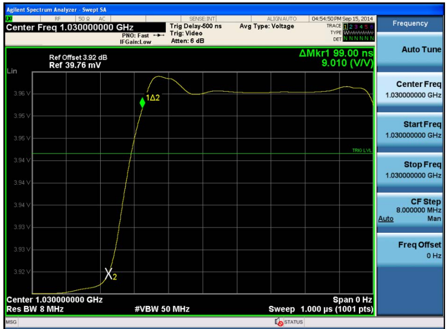
Figure 9-9: Rise time measurement of P1 pulse
