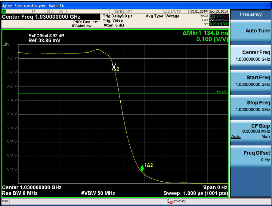
Figure 9-12: Fall time measurement of P3 pulse
