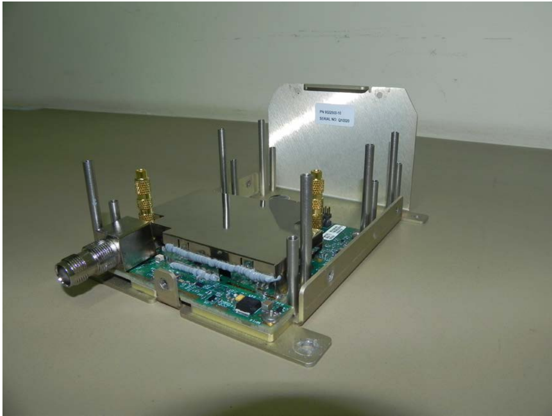
Figure 5-8: NGT-2500 with GPS-UAT CCA and Power Supply CCA Removed
