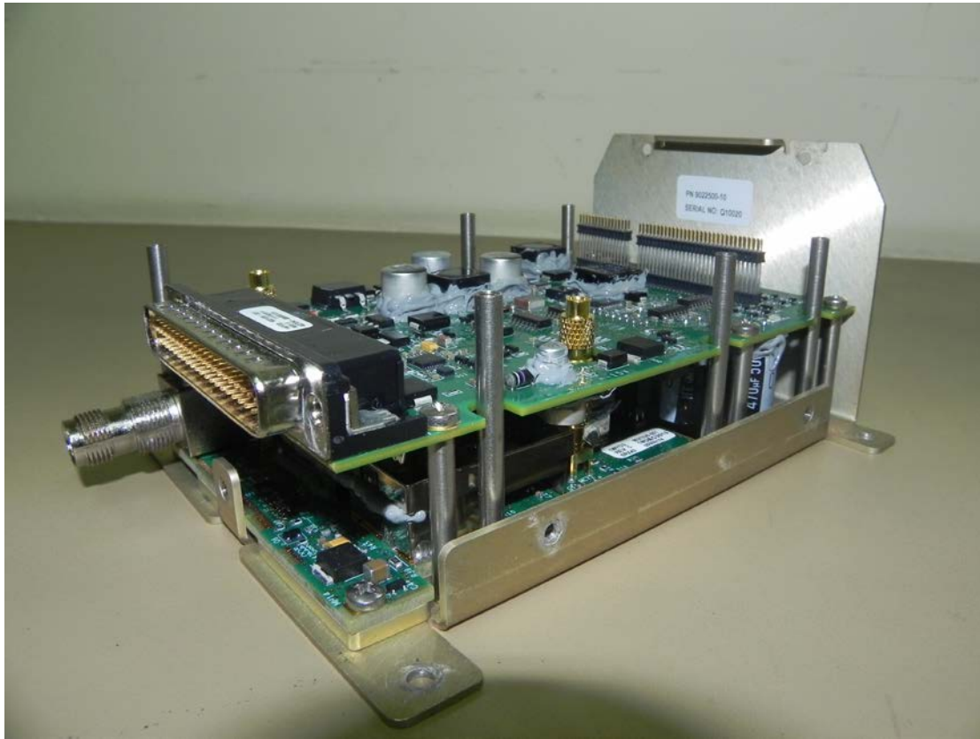
Figure 5-5: NGT-2500 with GPS-UAT CCA Removed
