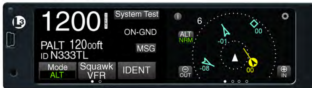
Figure 3-20: Example of Normal Operation
