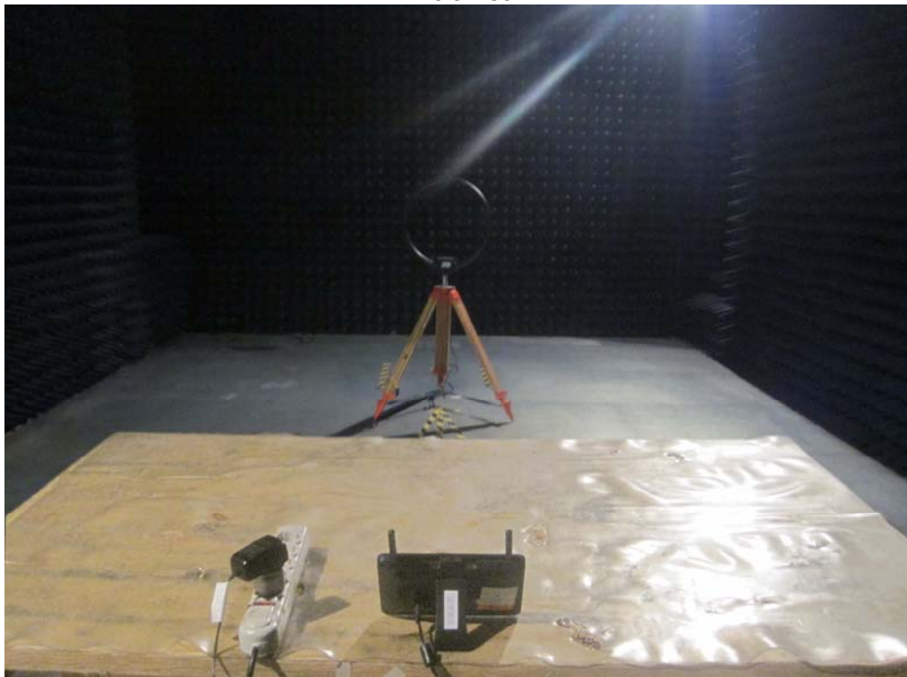
Photograph – Radiation Spurious Emission Test Setup
