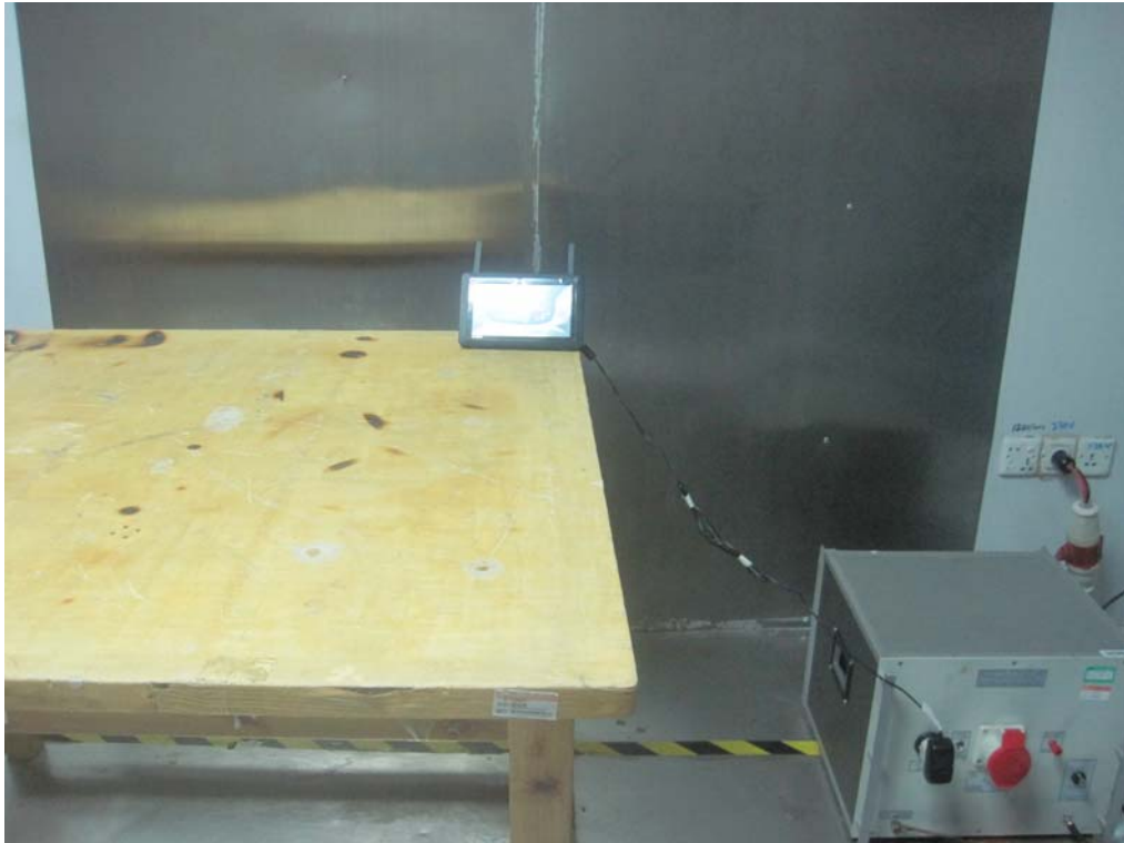
Photograph – Conducted Emission Test Setup
