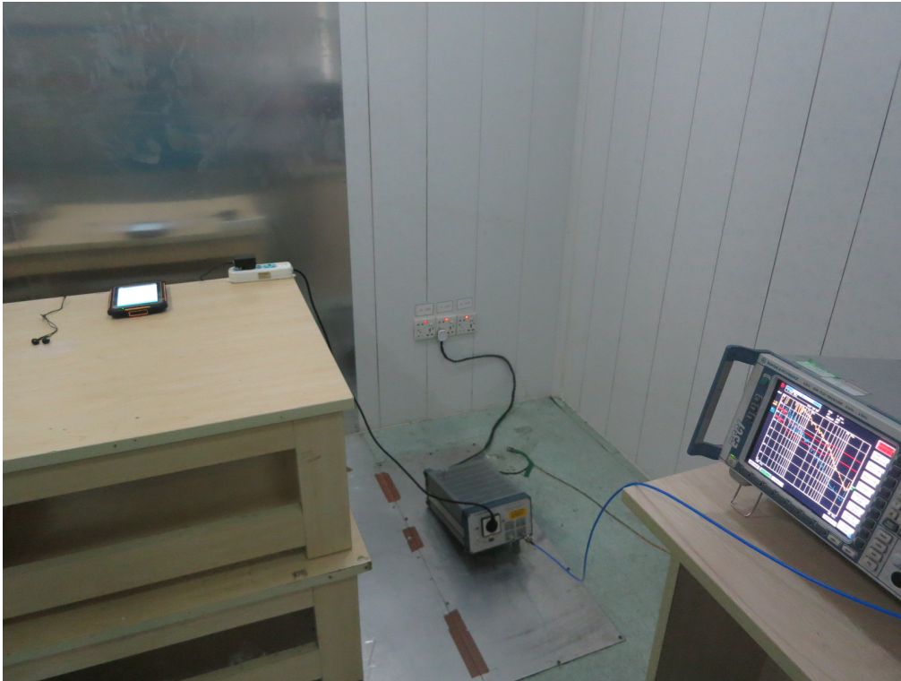
FCC LINE CONDUCTED EMISSION TEST SETUP
