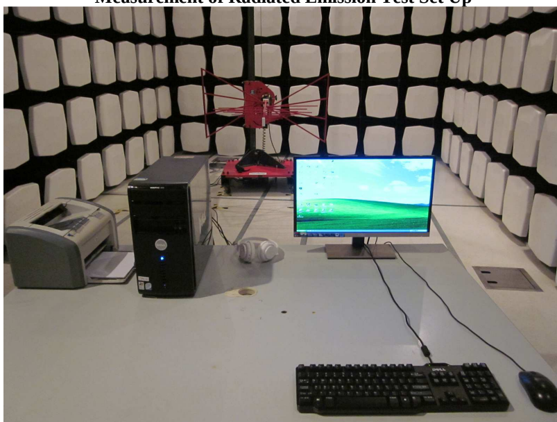
Measurement of Radiated Emission Test Set Up
