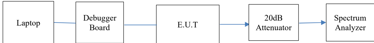
Figure 1. Configuration of Tested System Conducted
