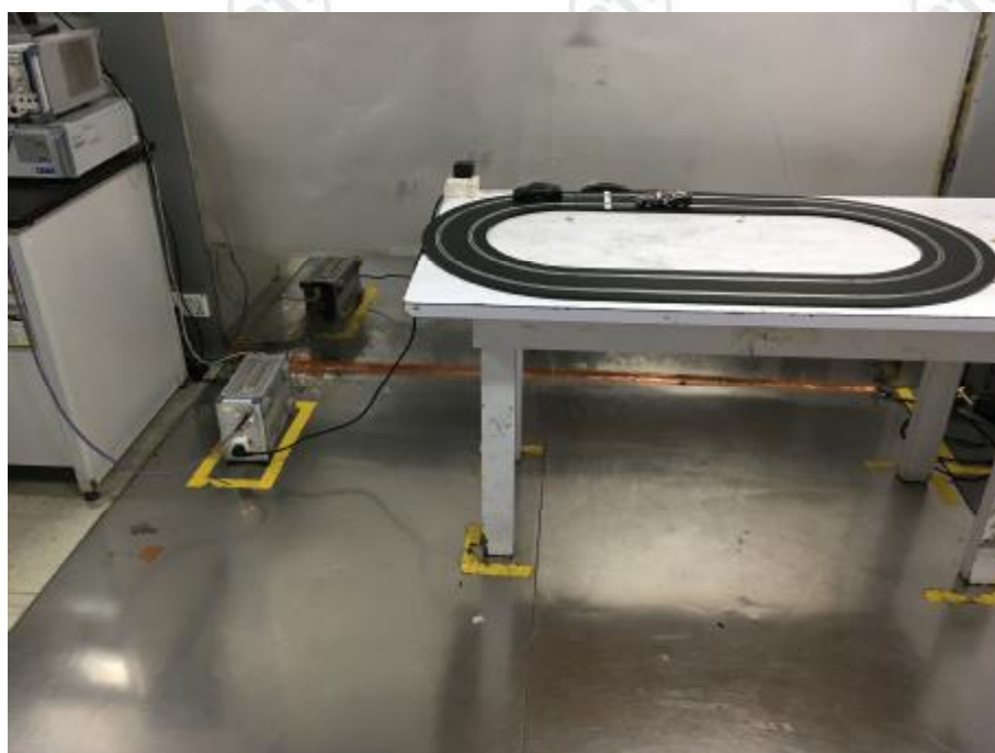
Conducted Emissions Test Setup
