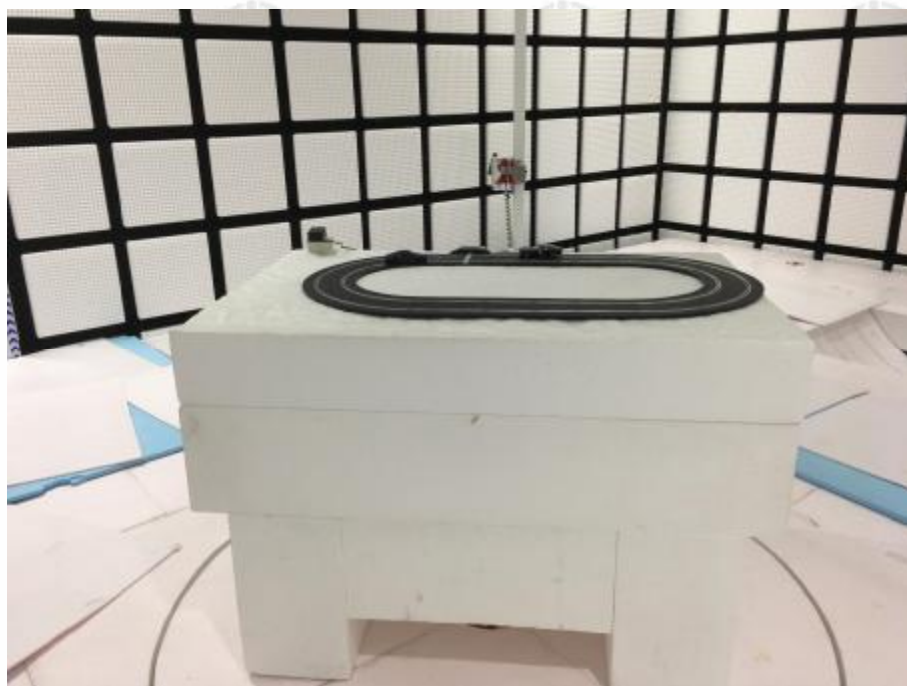
Radiated spurious emission Test Setup-3(Above 1GHz)
