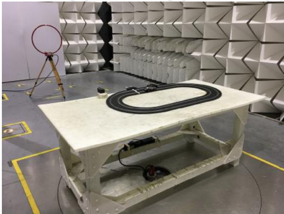
Radiated spurious emission Test Setup-1(Below 30MHz)
