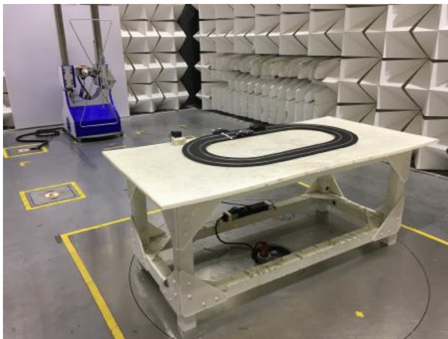
Radiated spurious emission Test Setup-2(30MHz-1GHz)
