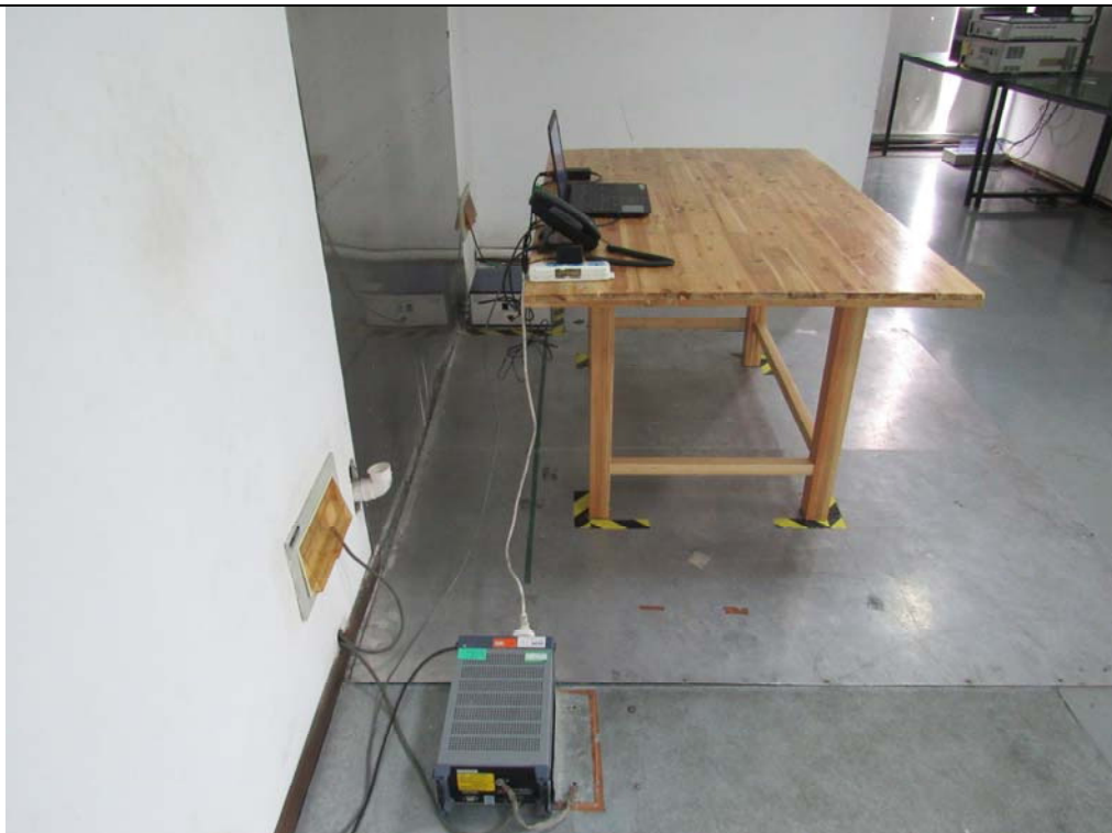
Conducted Emissions Setup Side View
