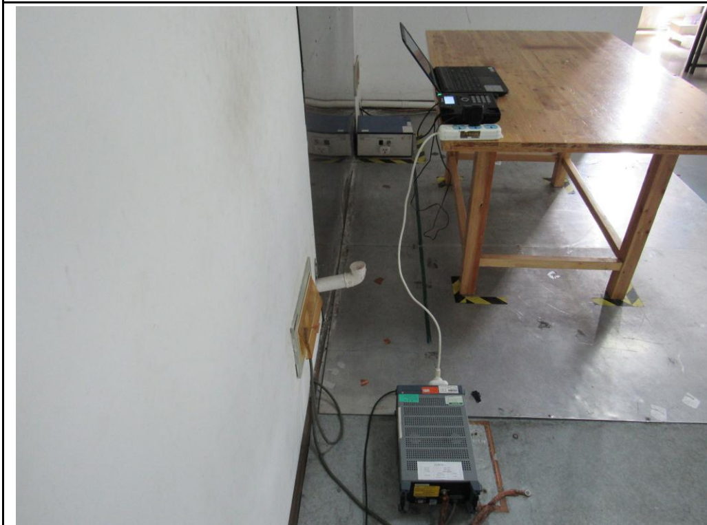
Conducted Emissions Test Setup Side View
