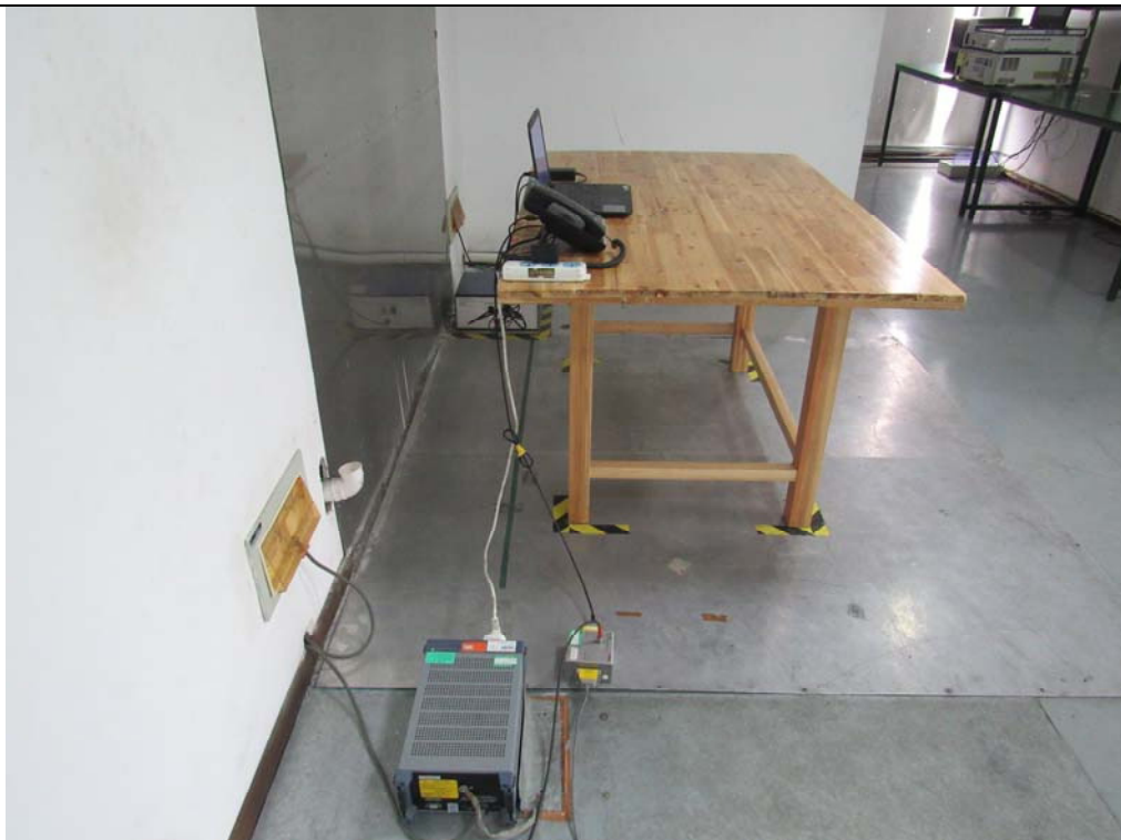
Conducted Emissions Setup Side View
