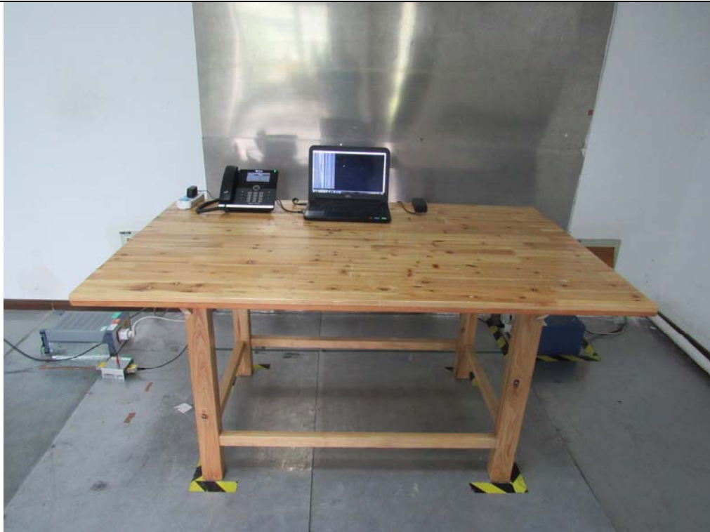
Conducted Emissions Setup Front View
