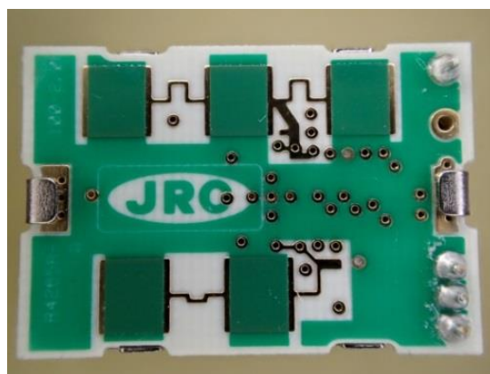
Front side: Patch Antenna
