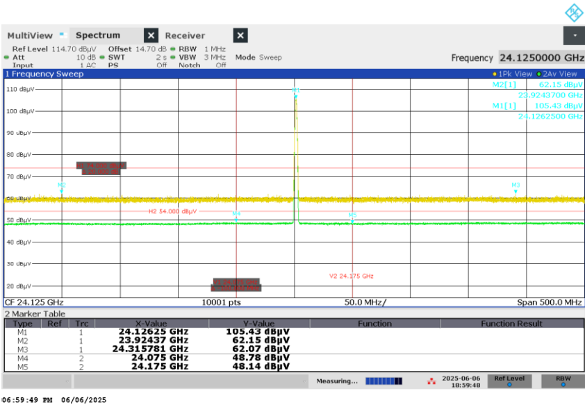
Figure 11: Radiated Emissions at Band Edge, Spectral Diagram, Mode A at Configuration 1
