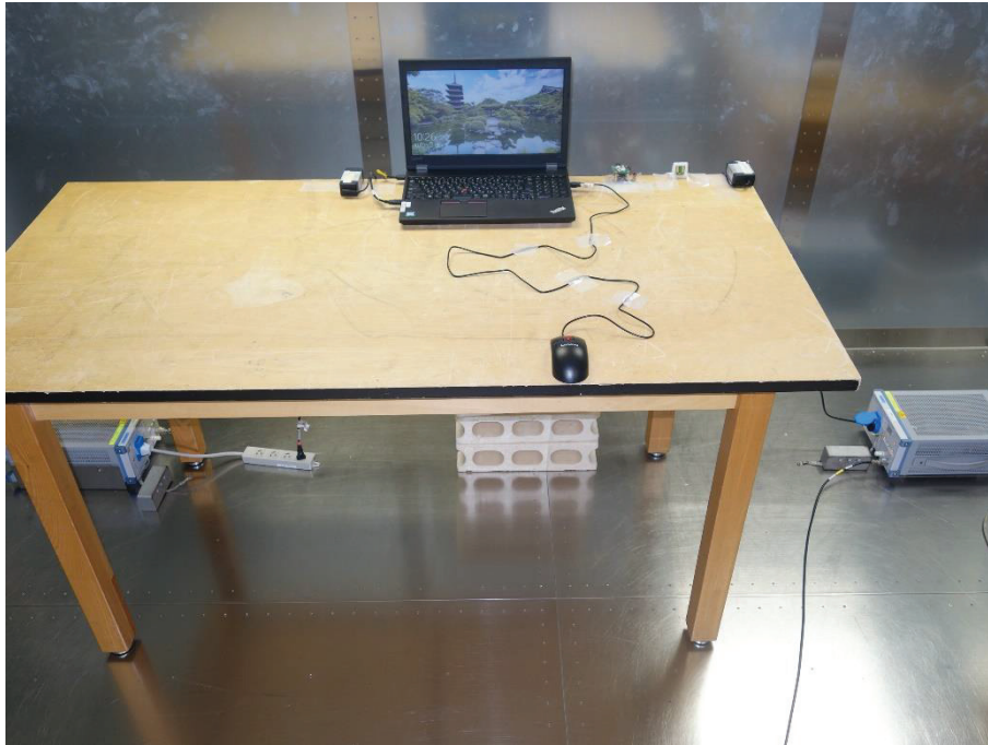
Photograph 1: Set-up for AC Power Line Conducted Emission, Front View
