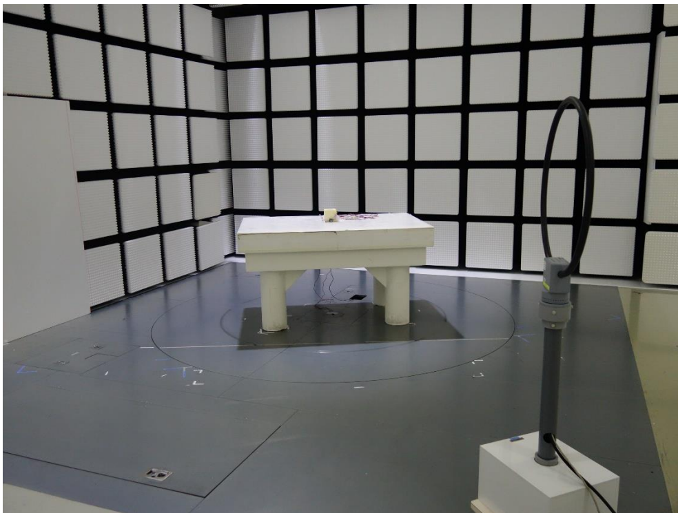
Photograph 8: Set-up for Radiated Emission below 30MHz, General View
