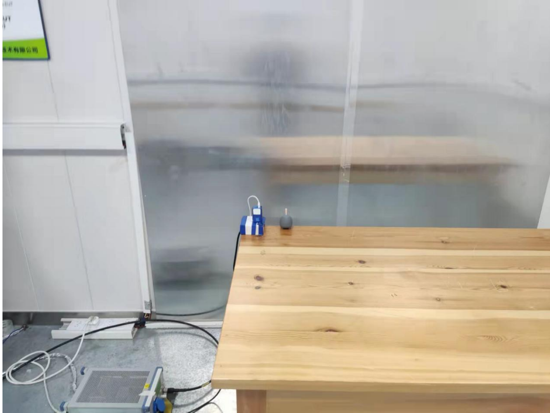
Conducted emission test setup
