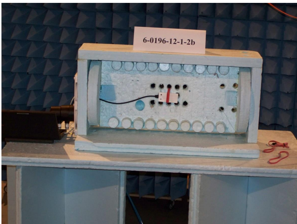
Radiated field strength measurements in the SAR (Semi-Anechoic-Chamber)
