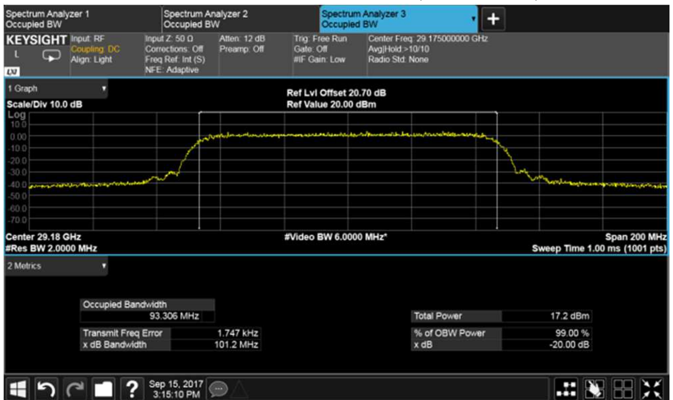
Plot for 99 % Bandwidth (MHz) Nominal Temp & Volts
