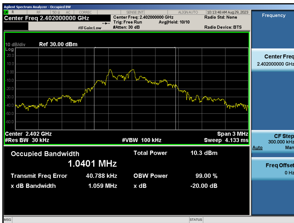
TEST PLOT OF BANDWIDTH FOR LOW CHANNEL
