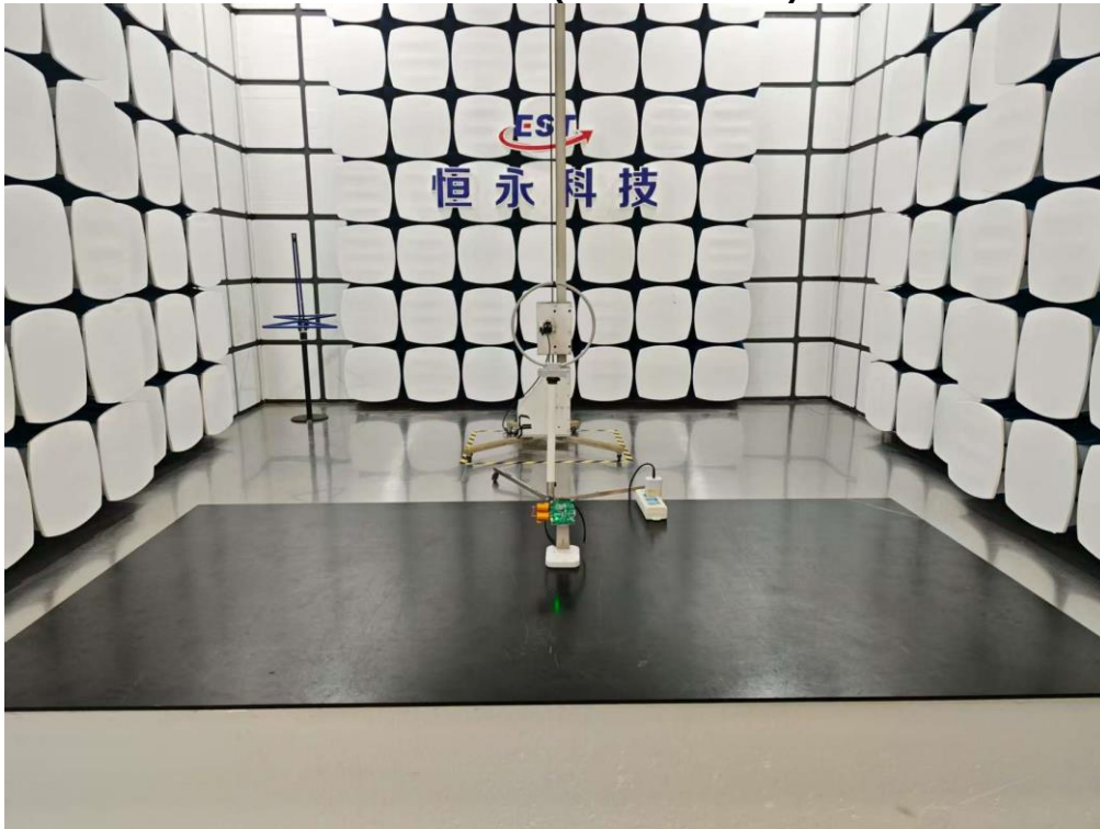
Radiated Test (Below 30MHz)
