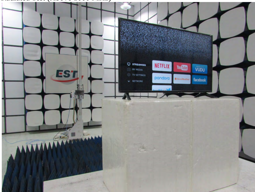
Radiated Test (Above 1000 MHz)
