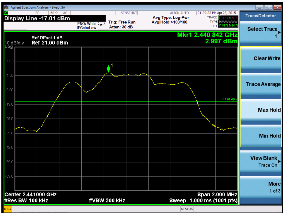
(Plot 4.7.2 B1: Channel 39: 2441MHz @8DPSK)
