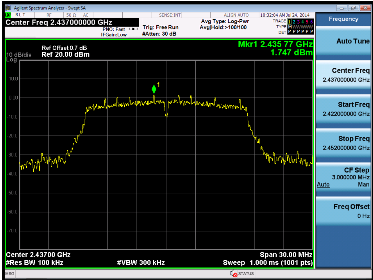
(Plot 4.6.2 B1: Channel 6: 2437MHz @ 802.11g)
