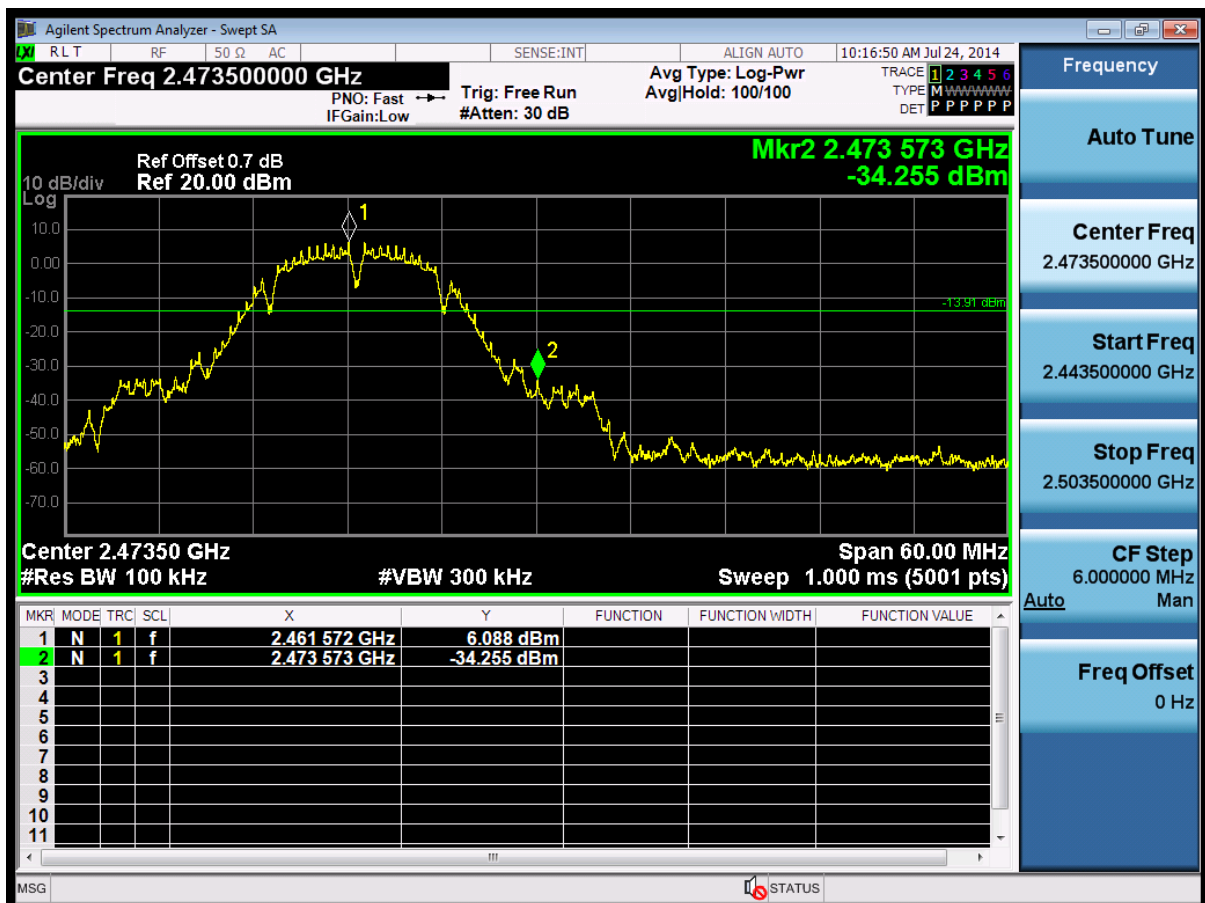
(Plot 4.6.1 C3: Channel 11: 2462MHz @ 802.11b)
