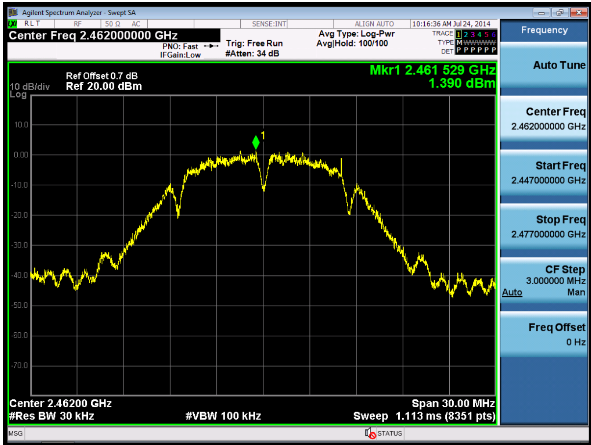
(Plot 4.4.1 C: Channel 11: 2462MHz @ 802.11b)
