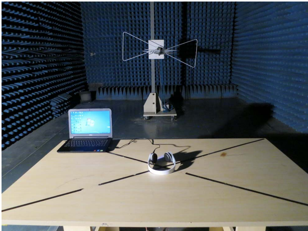
FCC RADIATED EMISSION TEST SETUP
