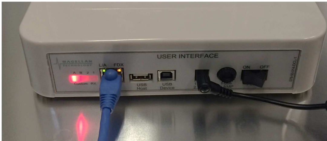
MDR-3021AT with power & Ethernet cables connected
