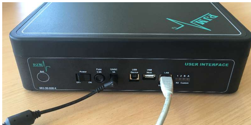
MDR-4330AT with power & Ethernet cables connected
