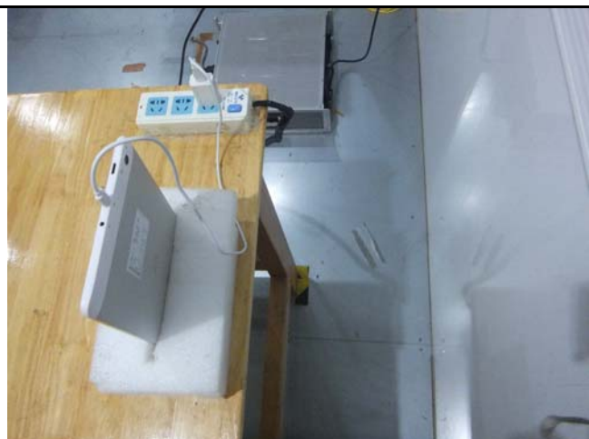
Conducted Emissions Test Setup Side View
