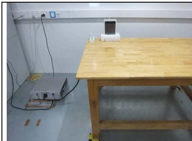
Conducted Emissions Test Setup Front View
