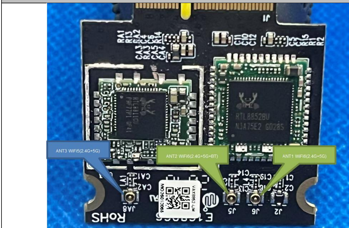
Antenna Ports Photo
