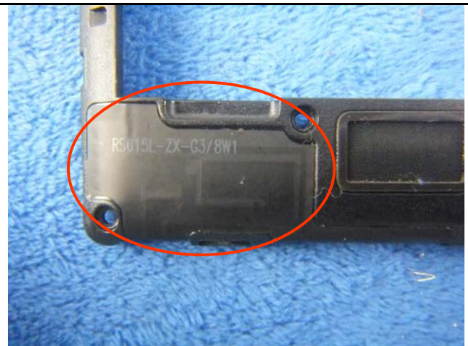
GSM/PCS/UMTS-FDD Antenna View
